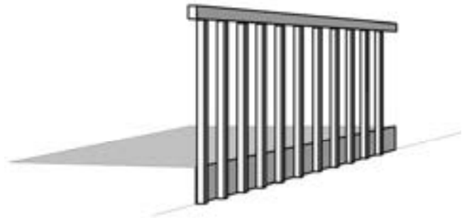
Figure A-1.2.2.B Cantilevered Picket System
